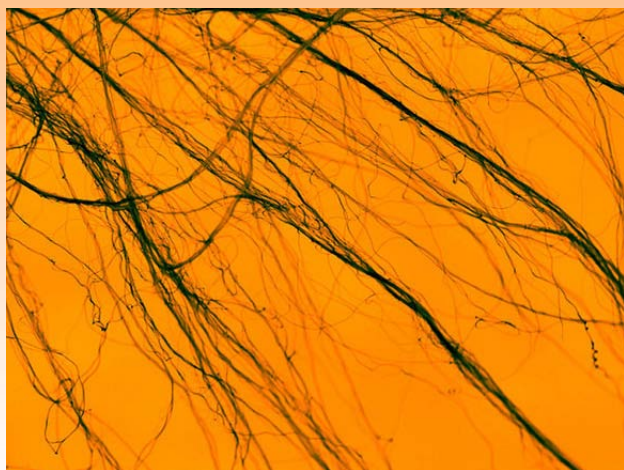
Carbon Nanotubes SEM micrograph of (multiwalled) carbon nanotube bundles (with false colour added). Magnification was about 7220x; the frame covers about 15 micrometres in the horizontal axis (1 micrometre = 1 millionth of a metre). The nanotubes themselves are roughly 10 nanometres (10 billionths of a metre) in diameter.
